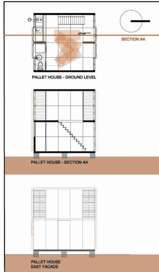
**Figure 8:** Plan, section and side elevation of PHS© Atacama case, coast of Iquique, Chile. Source: Suau.
