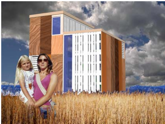
Figure 7: Rendering of PHS© Mediterranean case, outskirts of Barcelona (nearby Cerdanyola). The structure consists of a Euro-pallet frame, based on 120cm times 80cm each board. It is oriented to south and has double skill. The outer envelope towards south is a whitened shading device. Source: Suau.
