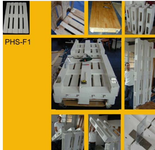
Figure 3: Structural test of PHS-F1© developed in my studio in Sweden. The whole structure consists of 8 Euro-pallet boards, collapsible and mobile. Its layout area is 80cm x 240cm. Source: Suau.
