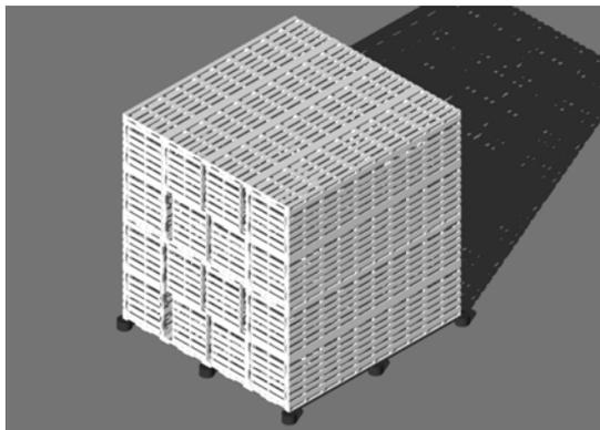
**Figure 1:** Rough 3D model of PHS© timber frame. The frame structure consists of Euro-pallet or US stringer boards, applicable in several contexts as roof, floors and wall framing and embraced mainly by plywood boards, tensile structures, etc. Source: Suau.
