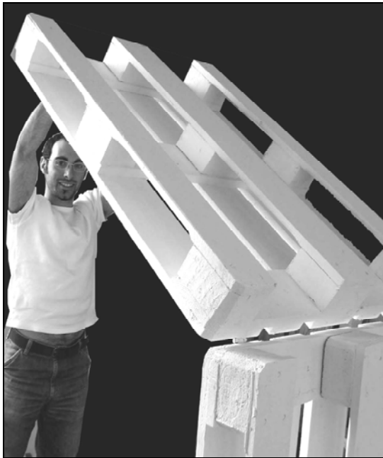
Figure 3: Structural test of PHS-F1© developed in my studio in 2004. The whole structure consisted of simulate the collapsible way to assemble a triangular chassis by using Euro-pallet boards. The TPH© roof is supported by a tensile V-bracing using two metal straps. Afterwards, the panels are reinforced by plywood boards on each deck. The unions of floor desk with lateral pitched roofs are executed with metal bins and joints. Source: Suau.
