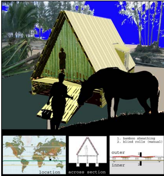
Figure 6: Rendering of TPH© Tropical case. It includes location, across section and climatic detail. The roofs and north-south façades contain both a movable shading device (bamboo logs) and internal roll blinds, which provide privacy. Source: Suau.
